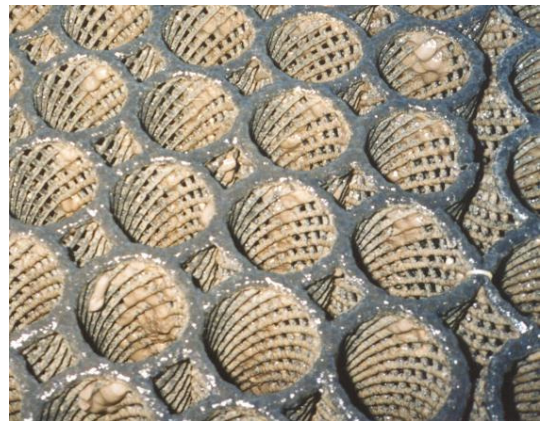
Biofilm developed on the surface of a BIO-BLOK ® media
